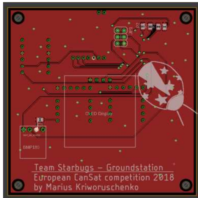
Figure 26: Receive PCB ground station top side
